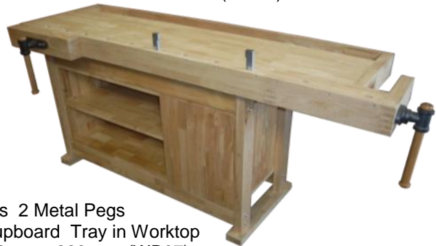
2 Vices High Shelf 3 Drawers 1 Cupboard 2 Metal Dogs Tray in 1260mm x 50mm x 840mm (WB03)
