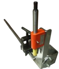
PIPE/TUBE NOTCHERS (TN2) are used with a power or hand drill to notch round or square pipe and tube. It uses standard hole saws up to 75mm. This can be performed at various angles from 0-45°.
